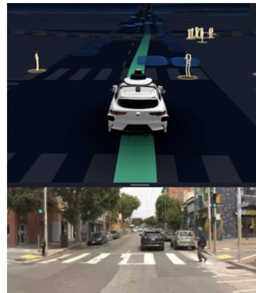
An AV detects a pedestrian in a crosswalk along with other pedestrians on the sidewalks
